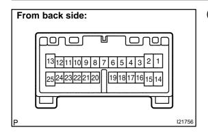
(c) Connect the connector to amplifier and inspect wire harness side connector from the back side, as shown in the chart below.
